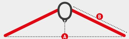
Measurement **A** is taken from shroud to shroud. Measurement **B** is taken from the mast groove to a straight line taken from shroud to shroud.
